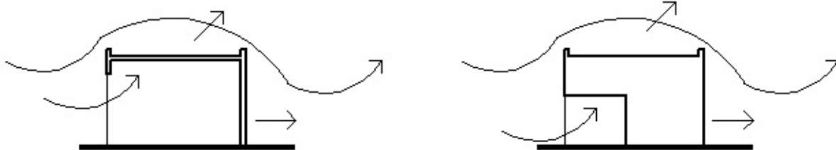
Figure 1. Partially enclosed buildings can cup the wind and increase pressures on the leeward side.
